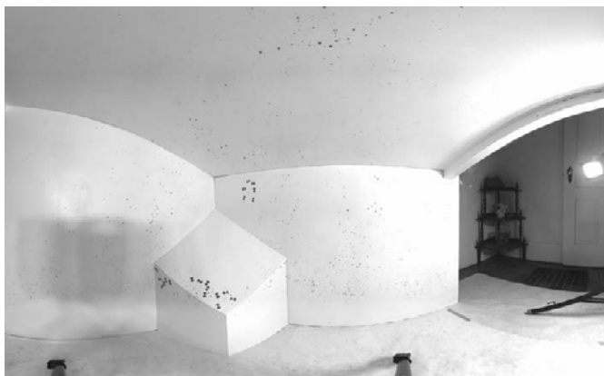
An example of a point cloud generated to give a three-dimensional representation of the area scanned, opened in the FARO Scene software.
